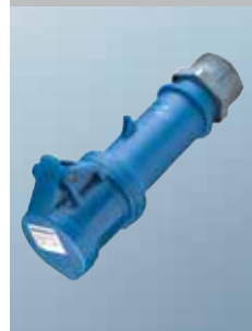
Connector ProTOP with screw terminals, cable gland and sealing, strain relief and protection against kinking, enclosure with thread lock and safety slide 16A, 3P, 230V
