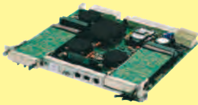
AdvancedTCA® carrier board with AdvancedMC™ modules
